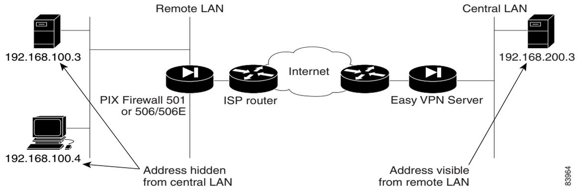
As shown in [Figure 4-2](#), client mode causes VPN connections to be initiated by traffic, so resources are only used on demand. In client mode, the PIX Firewall applies Network Address Translation (NAT) to all IP addresses of clients connected to the inside (higher security) interface of the PIX Firewall. To use this mode, you must also enable the DHCP server on the inside interface, as described in [“Using the PIX Firewall DHCP Server.”](#)
