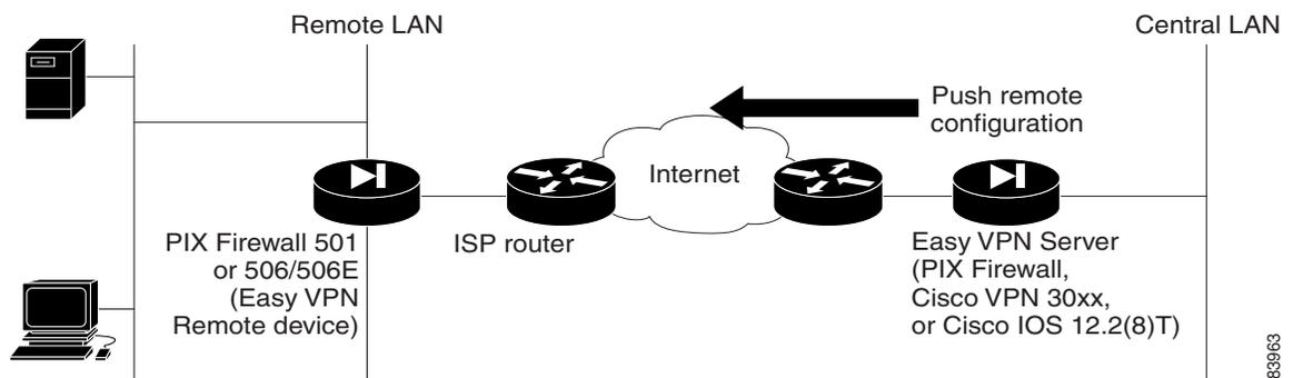
Easy VPN Remote device functionality, sometimes called a “hardware client,” allows the PIX Firewall to establish a VPN tunnel to the Easy VPN Server. Hosts running on the LAN behind the PIX Firewall can connect through the Easy VPN Server without individually running any VPN client software.
