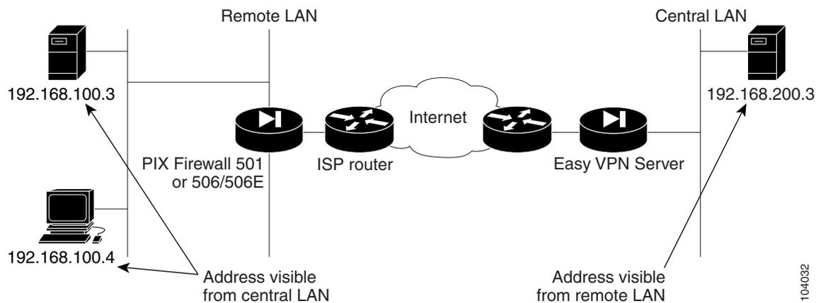
[Figure 4-3](#) illustrates network extension mode. In this mode, VPN connections are kept open even when not required for transmitting traffic. This option does not apply NAT to any IP addresses of clients on the inside (higher security) interface of the PIX Firewall.
